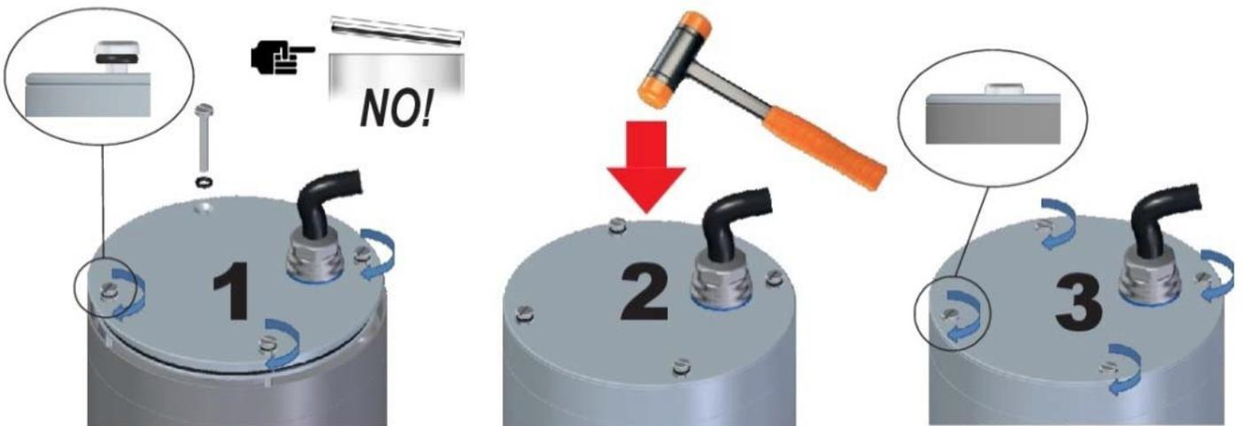
1. Slightly tighten the screws first (as delivered) before tightening them fully
